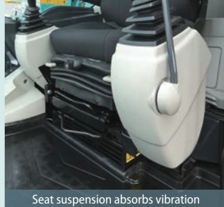
Seat suspension absorbs vibration
