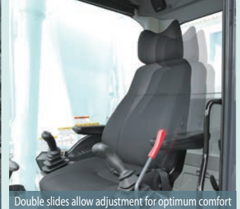
Double slides allow adjustment for optimum comfort
